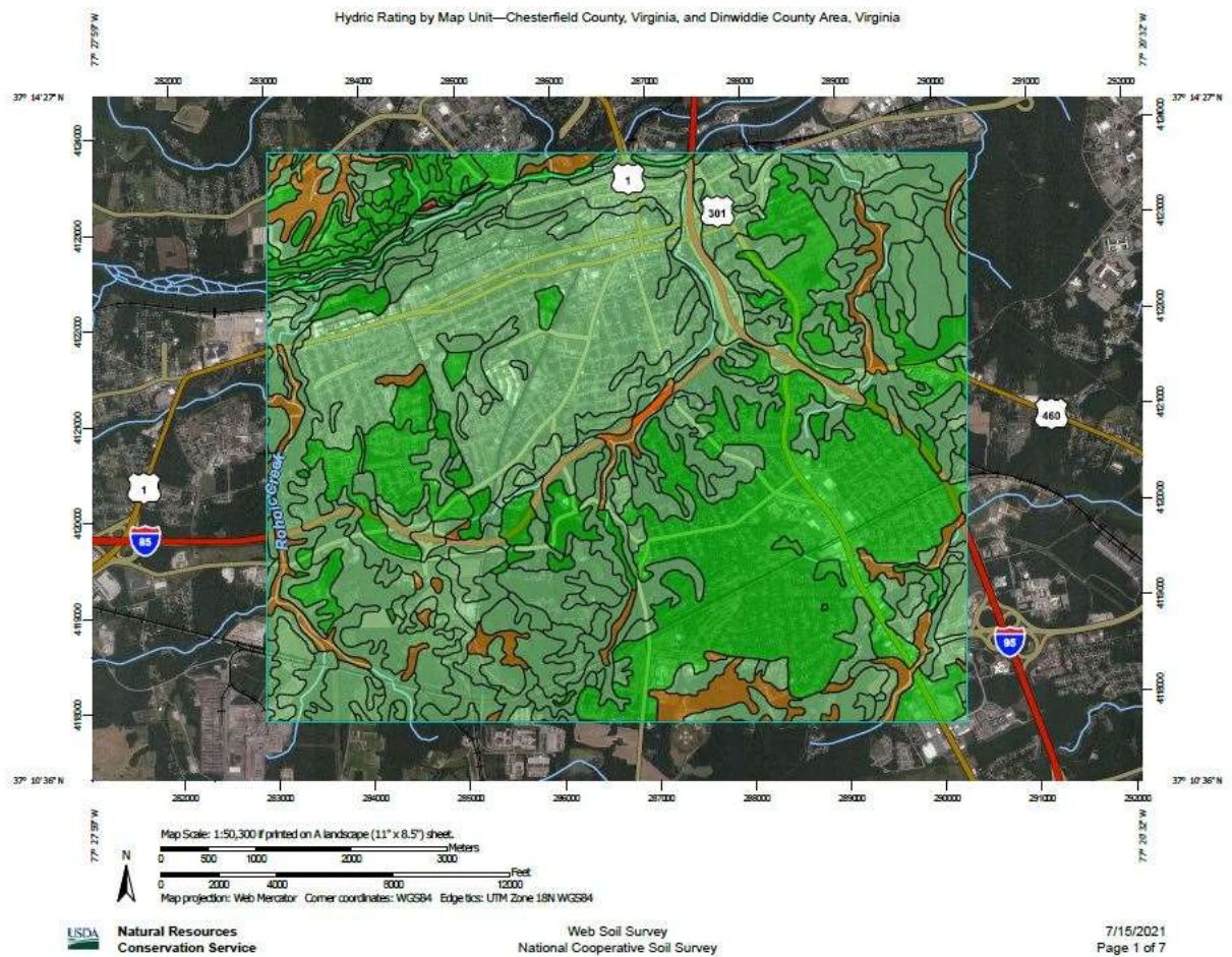
Map 7-5: Map showing the ability of the soil in the Greater Petersburg area to conduct water. Orange and red areas have the highest permeability, light green has the lowest. Note: Appomattox River is situated at the north side of the map, with Petersburg on the south bank
